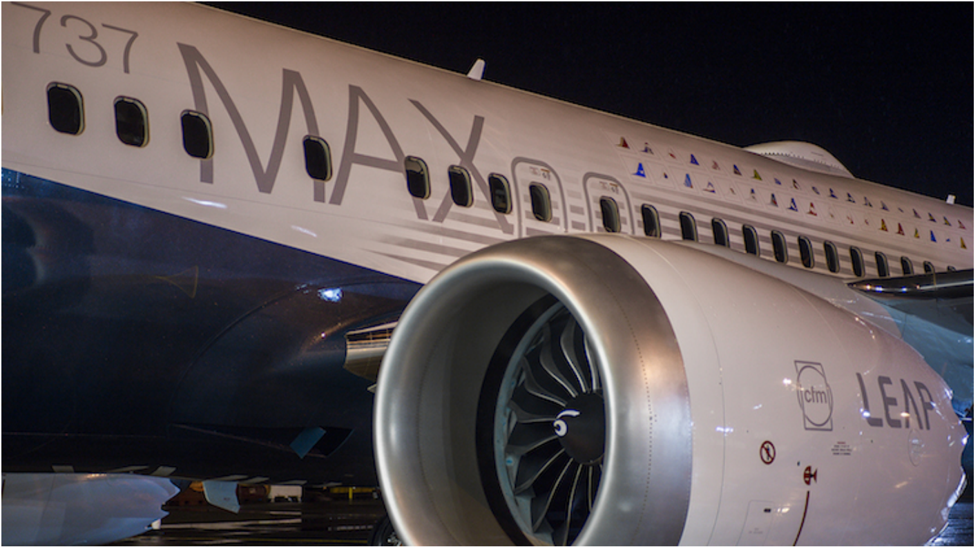
The 737 MAX is powered by two CFM International LEAP-1B engines. (Boeing)
