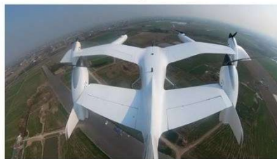
Transition by Tilting Rotors
